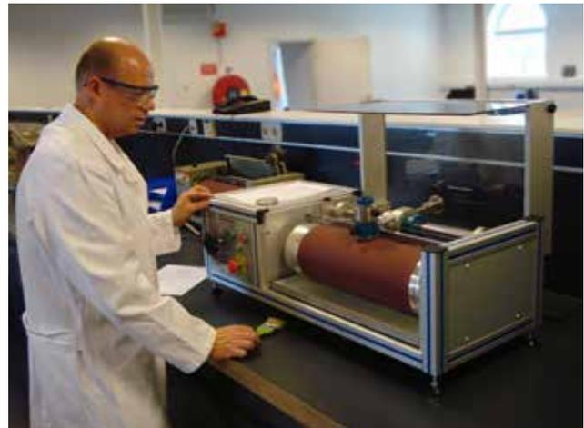
ISO 4649 / DIN 53516 abrasion testing.
